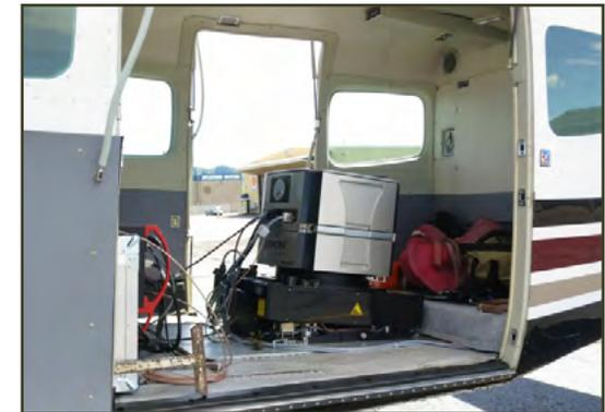
UltraCam Eagle installed in the aircraft.
