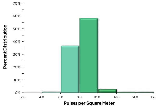
Average Pulse Density per 0.75' USGS Quad (color scheme aligns with density chart)
