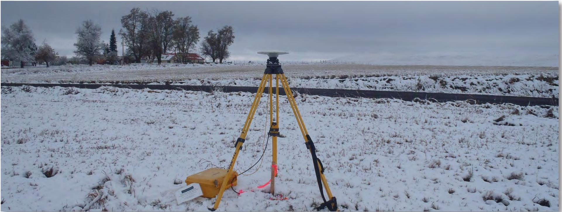
Base station set up over control "TURN\_03"
