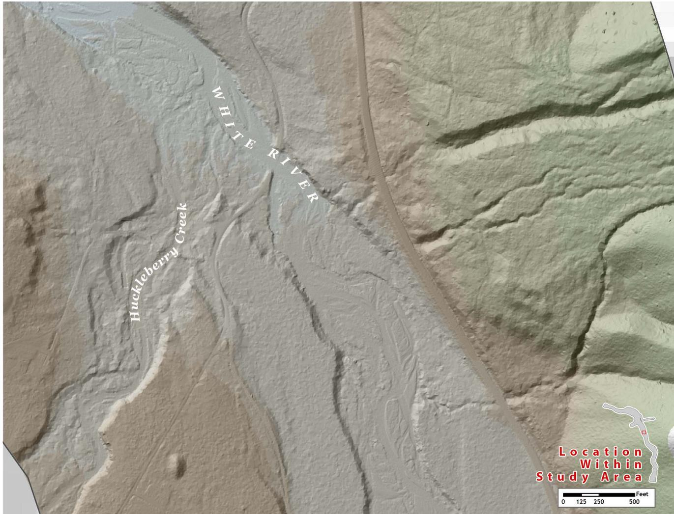
Figure 12. The Highest Hit Above Ground 3-foot resolution ESRI grid showing detail of Huckleberry Creek's confluence with the White River in the central portion of the SR410 Study Area. (To calculate vegetation heivalues shown in the map, the Bare Earth grid was subtracted from the Above Ground grid).
