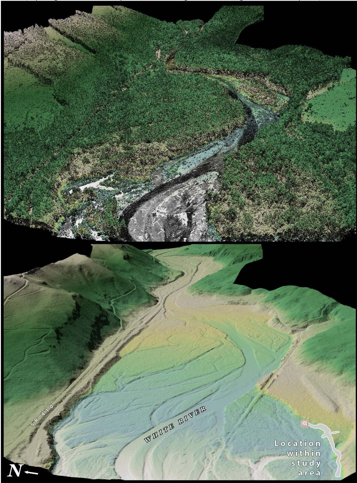
Figure 15. 3-d oblique view of LiDAR-derived surfaces in the southern portion of the SR410 Study Area. (Top image derived from all points, bottom image derived from ground-classified points).
