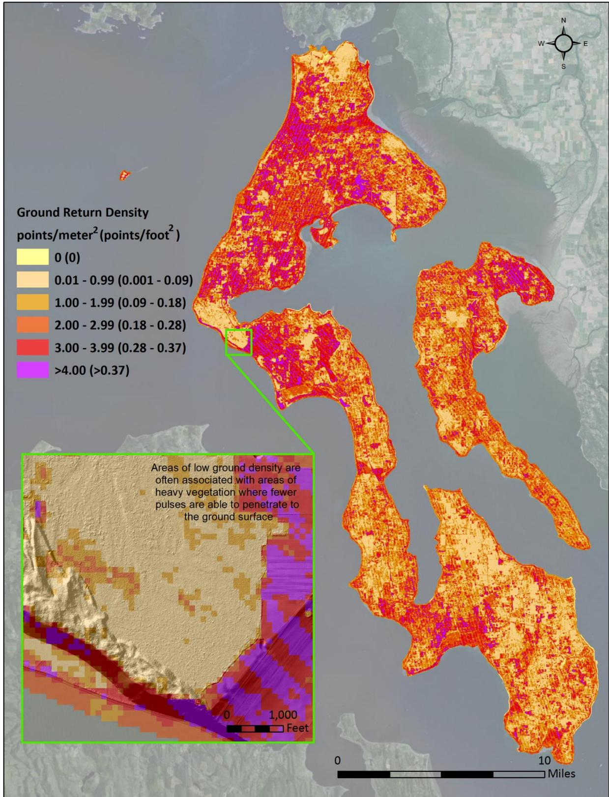
Figure 7: Ground density map for the Island County site (30 m x 30 m cells)
