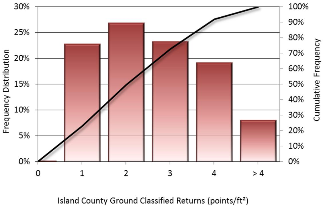
**Figure 5: Frequency distribution of ground return densities per 30 x 30 m cell**
