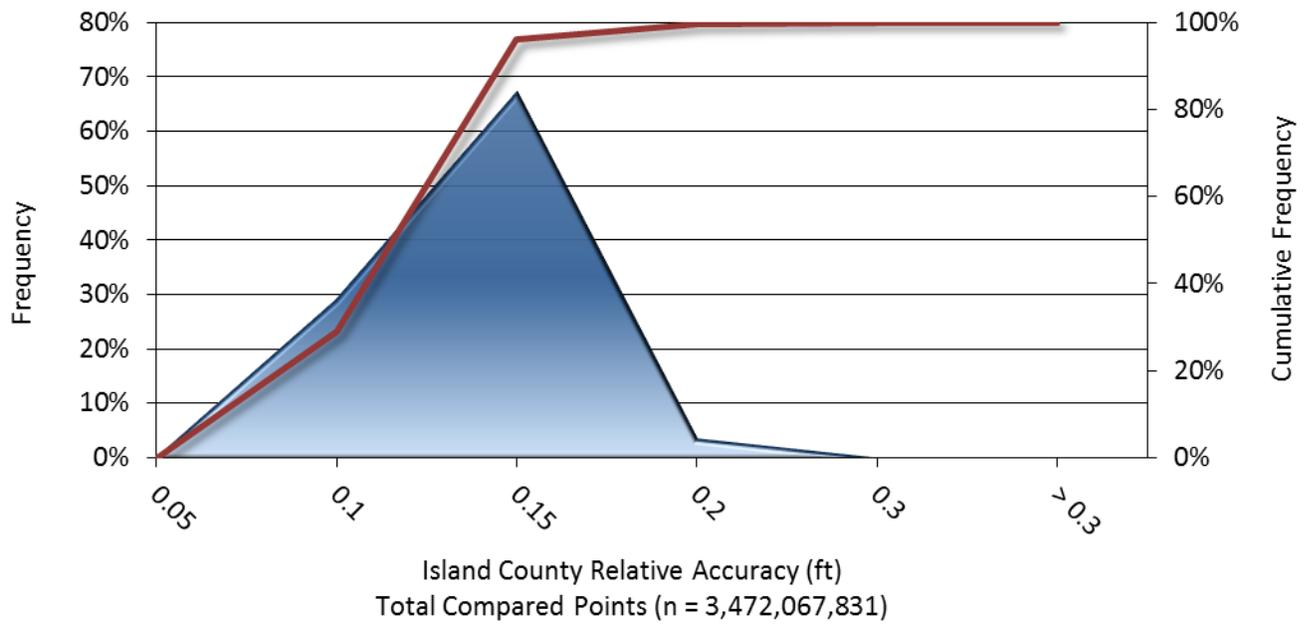
**Figure 9: Frequency plot for relative vertical accuracy between flight lines**
