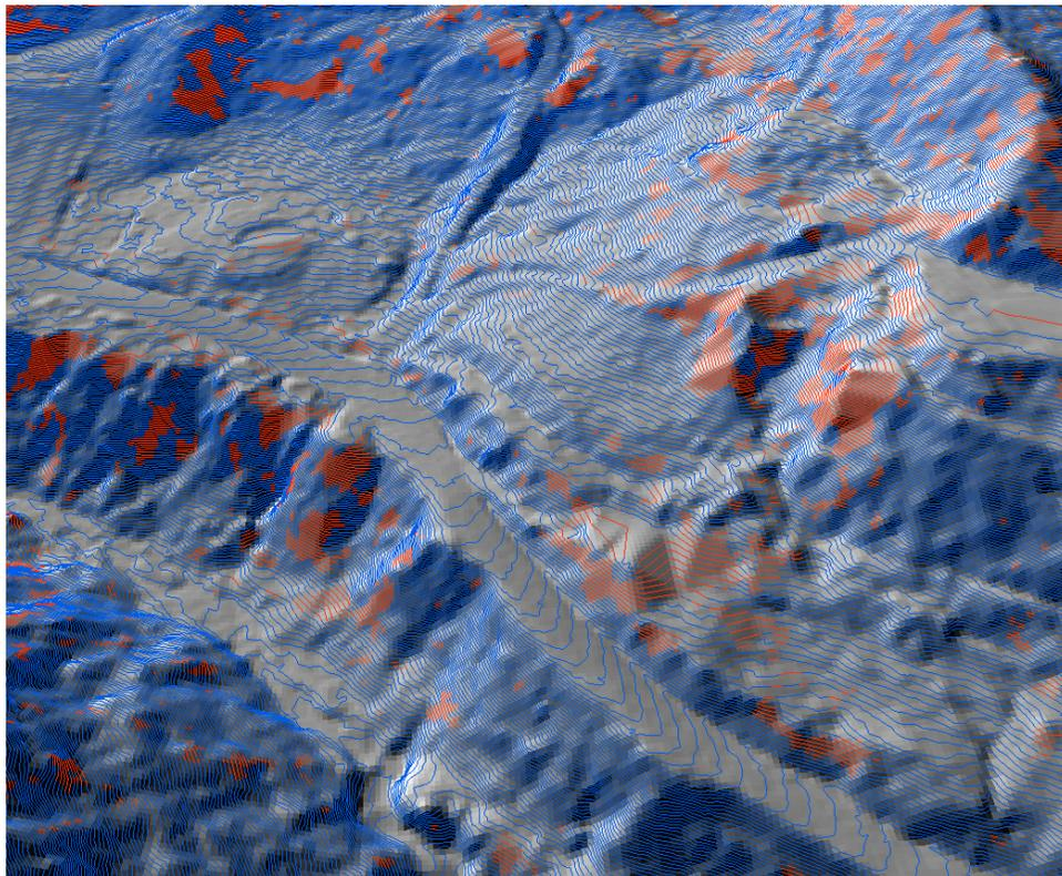
**Figure 3: Contours draped over the Island County bare earth elevation model. Blue contours represent high confidence while the red contours represent low confidence.**
