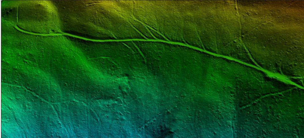
Figure 16: Temporary creation of TIN over ground points to assist in identifying points incorrectly classified as ground.
