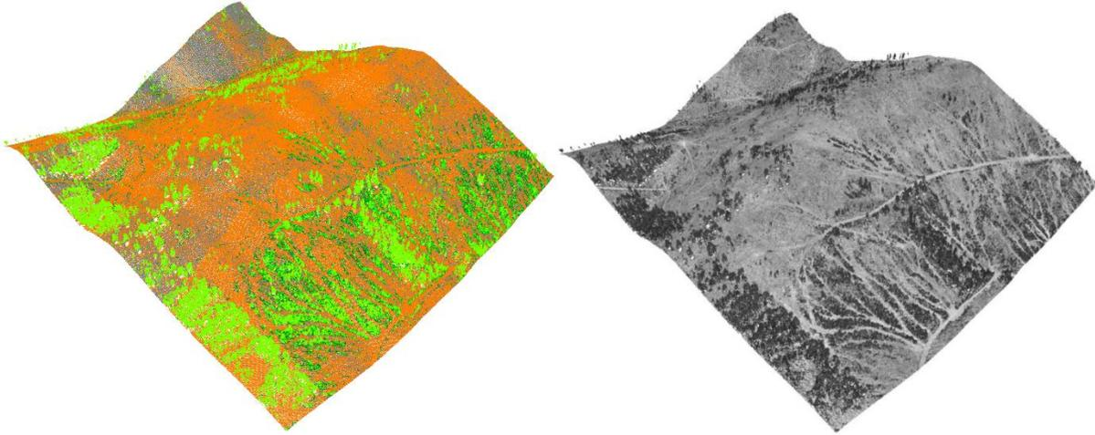
Figure 14: elected boxes of rotating 3D point clouds, viewed with toggled color-coded classification points
