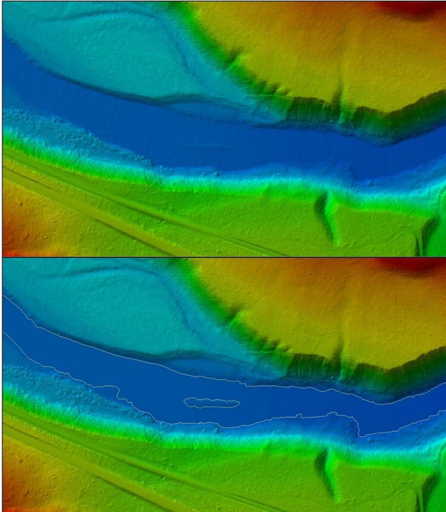
Figure 17: TIN Surface before implementing hydro breaklines enforcement and afterwards
