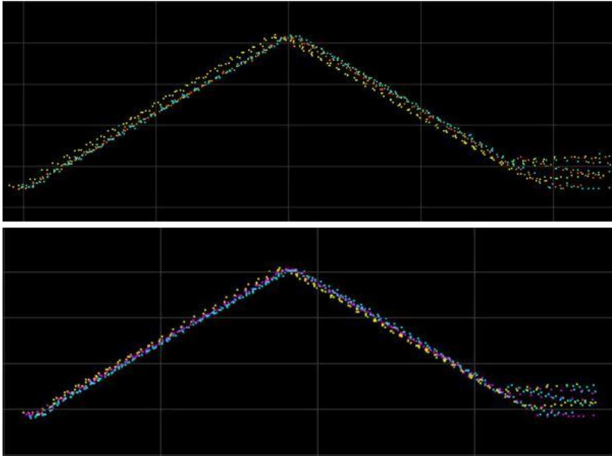
Figure 5: Planes in overlapping strips before and after adjustment
