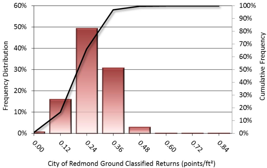
**Figure 4: Frequency distribution of ground return densities per 30 x 30 m cell**
