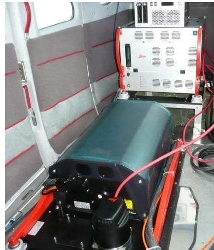
**Leica ALS70 LiDAR sensor**
