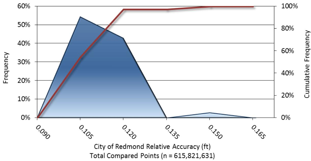
**Figure 8: Frequency plot for relative vertical accuracy between flight lines**
