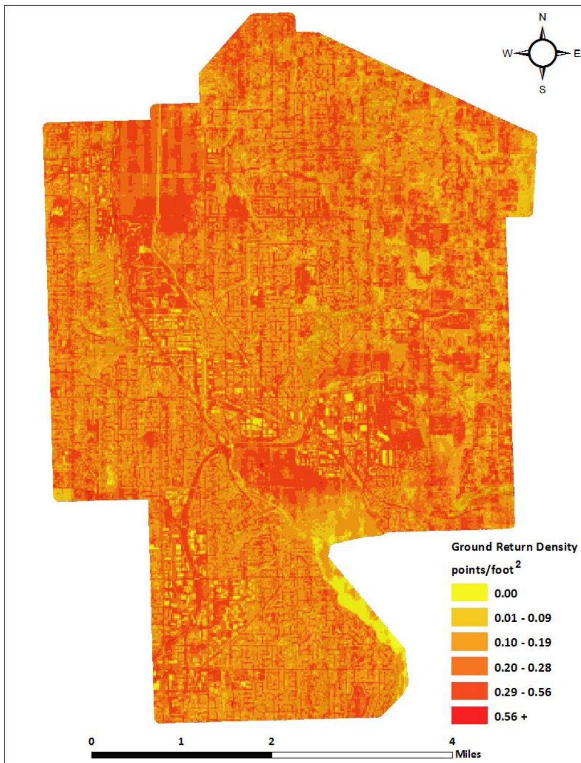
Figure 6: Ground density map for the City of Redmond site (30 m x 30 m cells)
