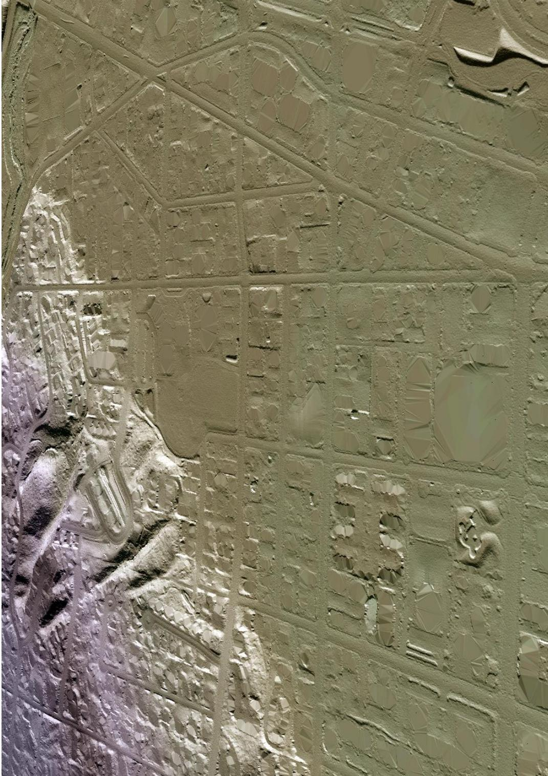
**Figure 9: View looking west over downtown Redmond. The image was created from the bare earth LiDAR model colored by elevation.**
