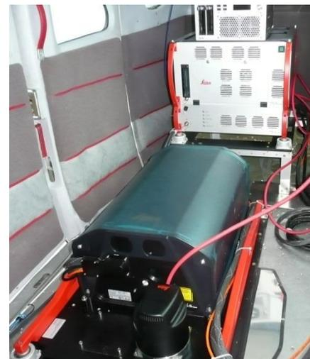
**Leica ALS70 LiDAR sensor**
