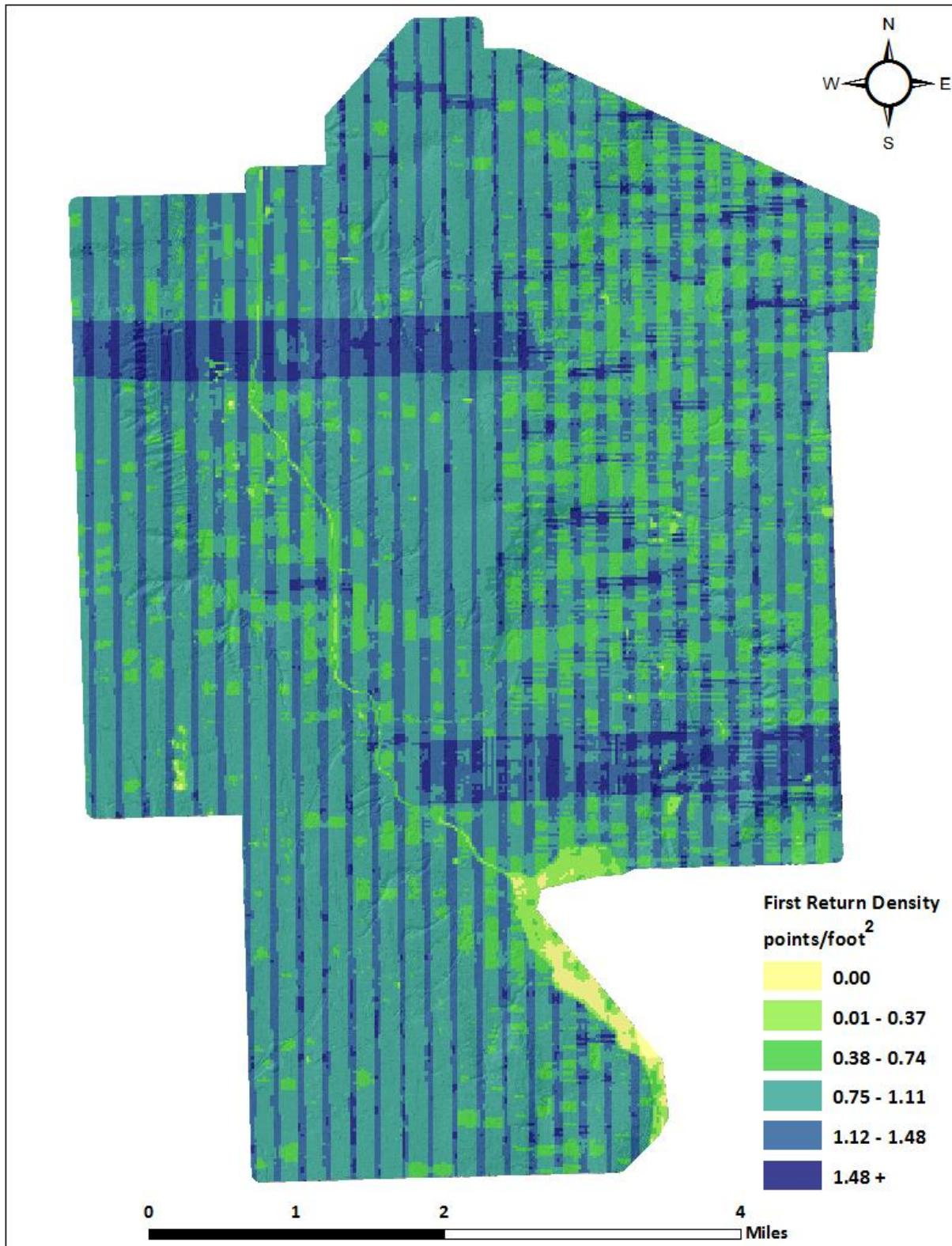
Figure 5: First return density map for the City of Redmond site (30 m x 30 m cells)
