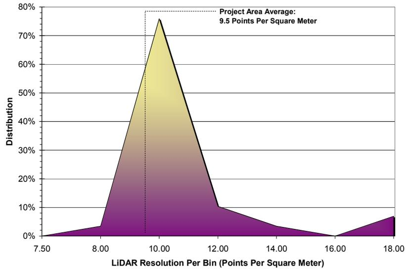
Figure 10. Image shows first return laser point data density in the Sumpter AOI, per processing bin.
