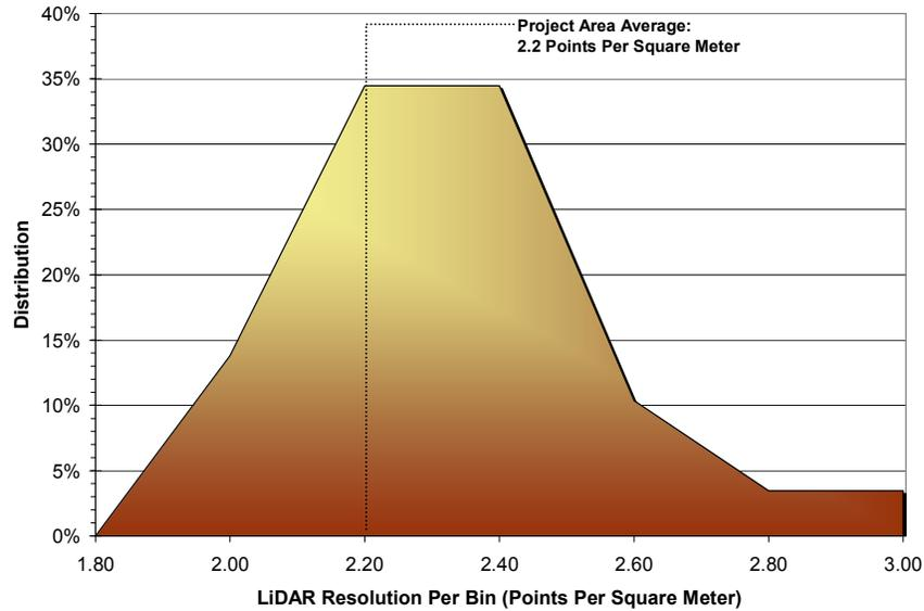
**Figure 12.** Image shows ground-classified laser point data density in the Sumpter AOI, per processing bin.
