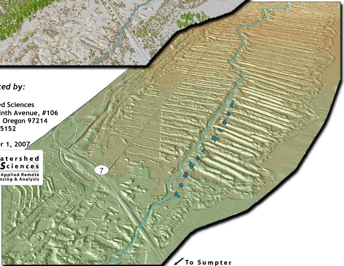
Study area east of Highway 7 shown in oblique view: top image is 1-meter resolution Above Ground ESRI Grid, bottom image is 1-meter resolution Bare Ground ESRI Grid.
