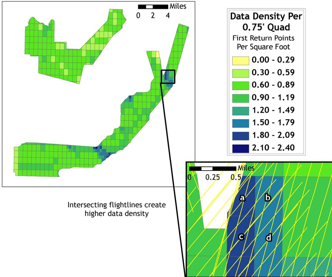
Areas containing water bodies produce lower first return point density. In delivery 4, low pulse densities coincide with Mayfield Lake in Lewis County (see Figure 4.12 below).
