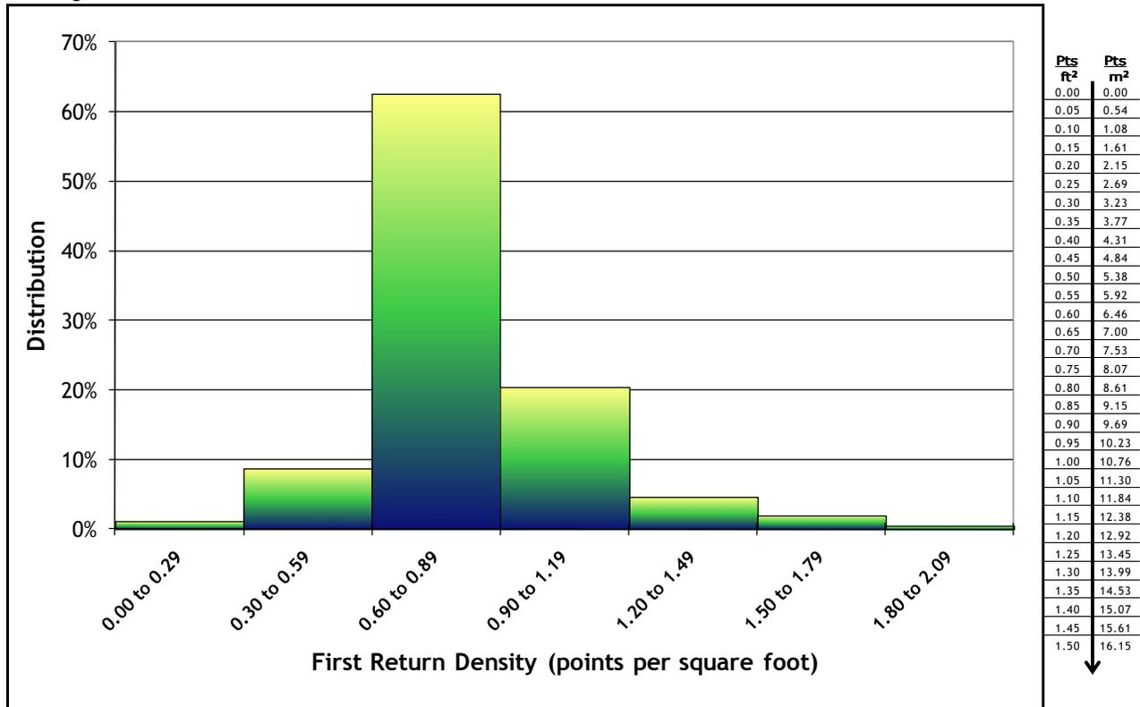
Figure 4.8. Image shows first return laser point density for in the Lewis County study area, per 0.75' USGS Quad.
