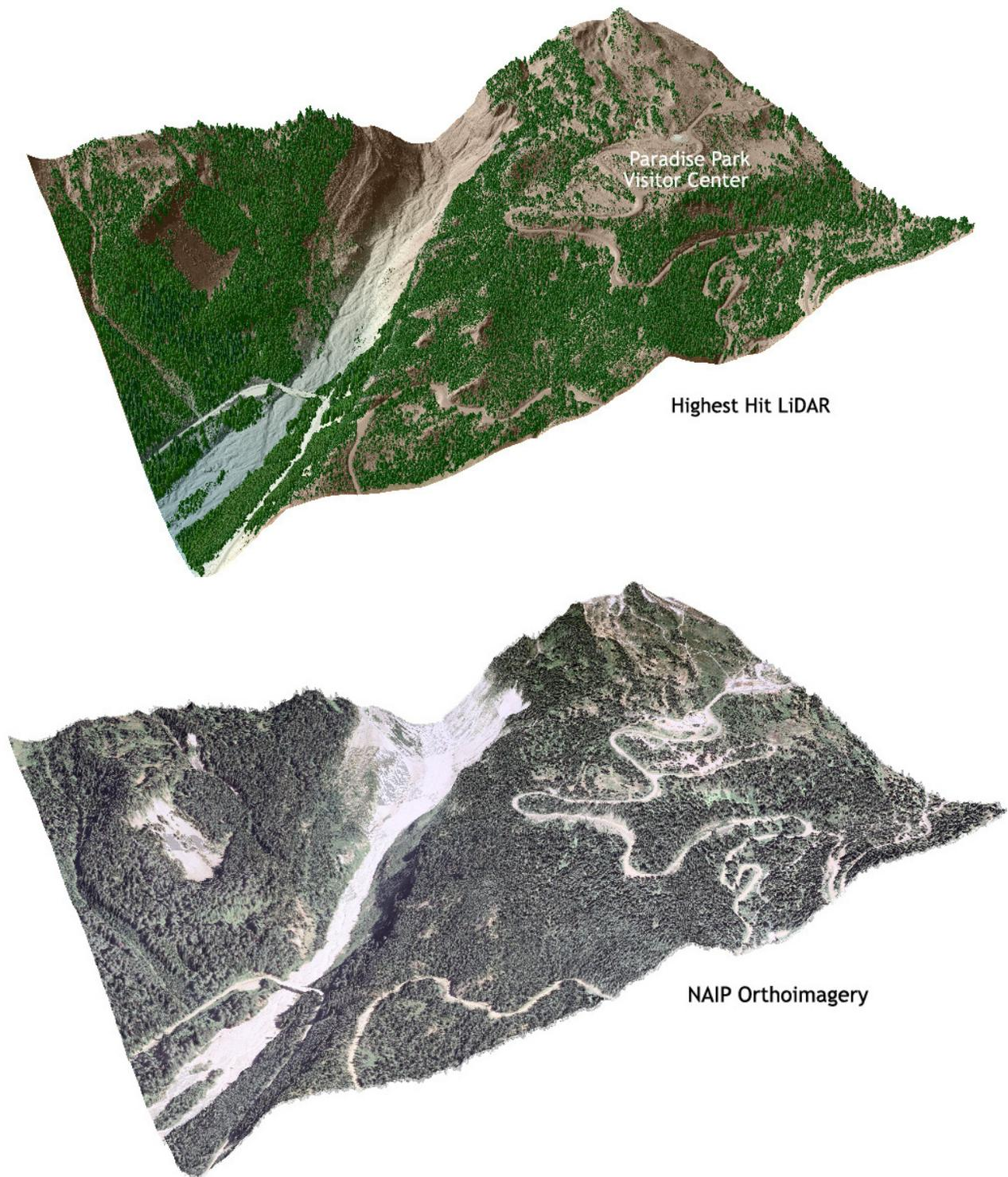
**Figure 8.6.** 3-d oblique view of Mineral, Washington, looking south-west over Mineral Lake (top image is derived from highest-hit classified lidar points, the bottom image is derived from ground-classified LiDAR points).
