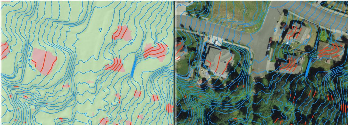
The CAD files (\*.DWG) are coded to display high and low confidence contours as green and red, respectively (**Figure 3.2**). The elevation label units are feet.
