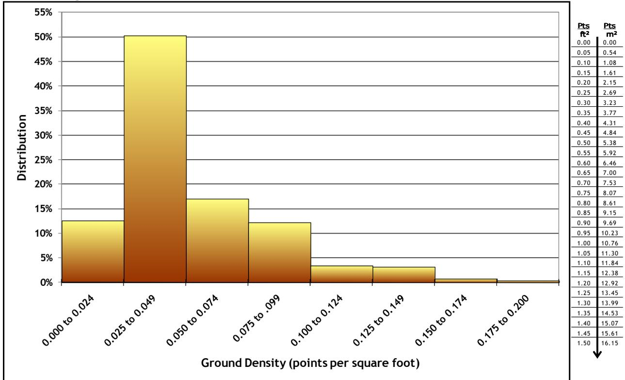
Figure 4.10. Image shows ground-classified laser point density for in the Lewis County study area, per 0.75' USGS Quad.
