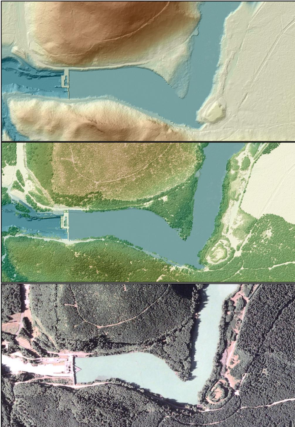
**Figure 8.8** 3-d oblique north-east view of the Cispus River, Washington (top image is derived from an orthophoto draped on the highest-hit model, middle image is a highest-hit model, the bottom image is derived from ground-classified LiDAR points).
