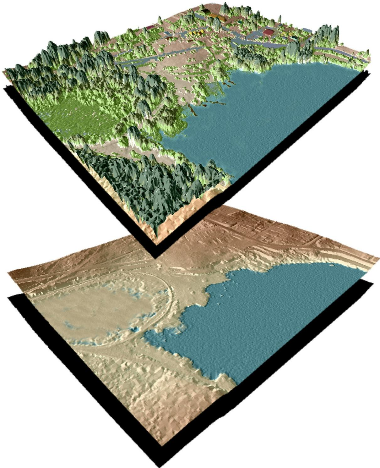
**Figure 8.7.** Plan view showing the Cowlitz River, the Cowlitz Falls Dam and Lake Scanewa (top image is derived from ground-classified LiDAR points, middle image is derived from highest hit classified LiDAR points and bottom image is an orthophoto).
