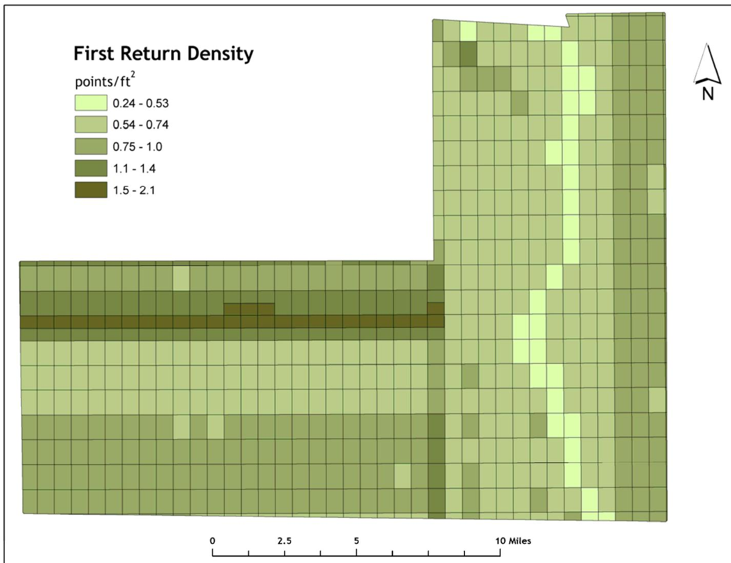
Figure 6. Ground density by 1/100<sup>th</sup> USGS tile
