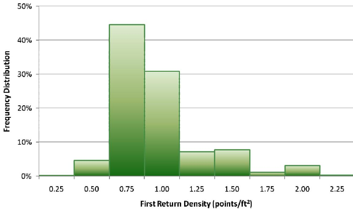
Figure 4. Density distribution for ground classified laser points.
