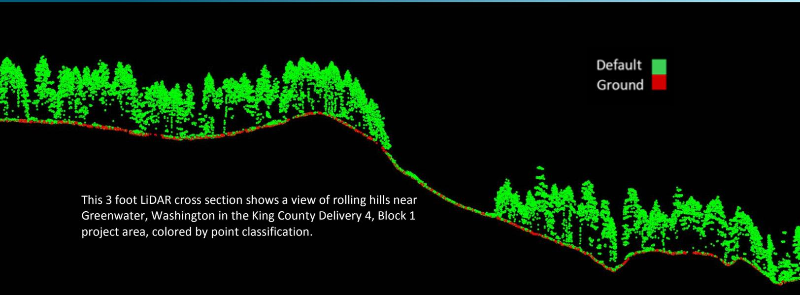
This 3 foot LiDAR cross section shows a view of rolling hills near Greenwater, Washington in the King County Delivery 4, Block 1 project area, colored by point classification.
