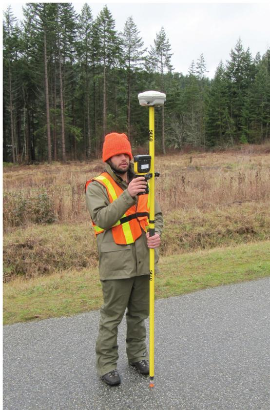
A WSI Ground Professional collects RTK points with a roving R8 unit.
