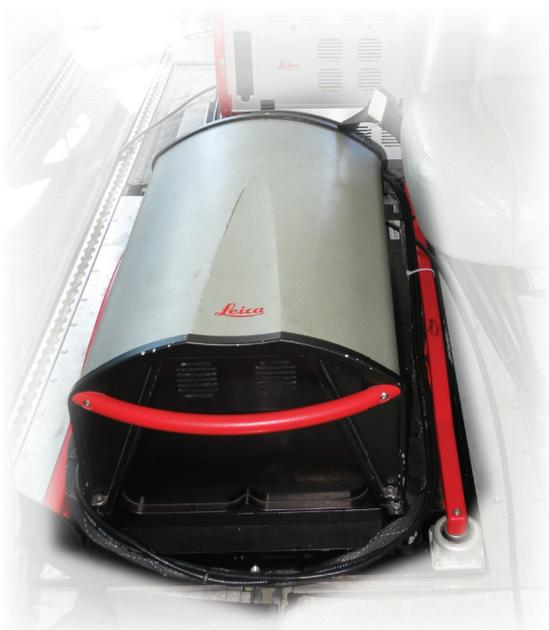
Leica sensor ALS 6106 installed in the aircraft
