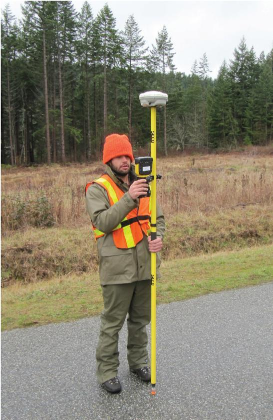
A WSI Ground Professional collects RTK points with a roving R8 unit.
