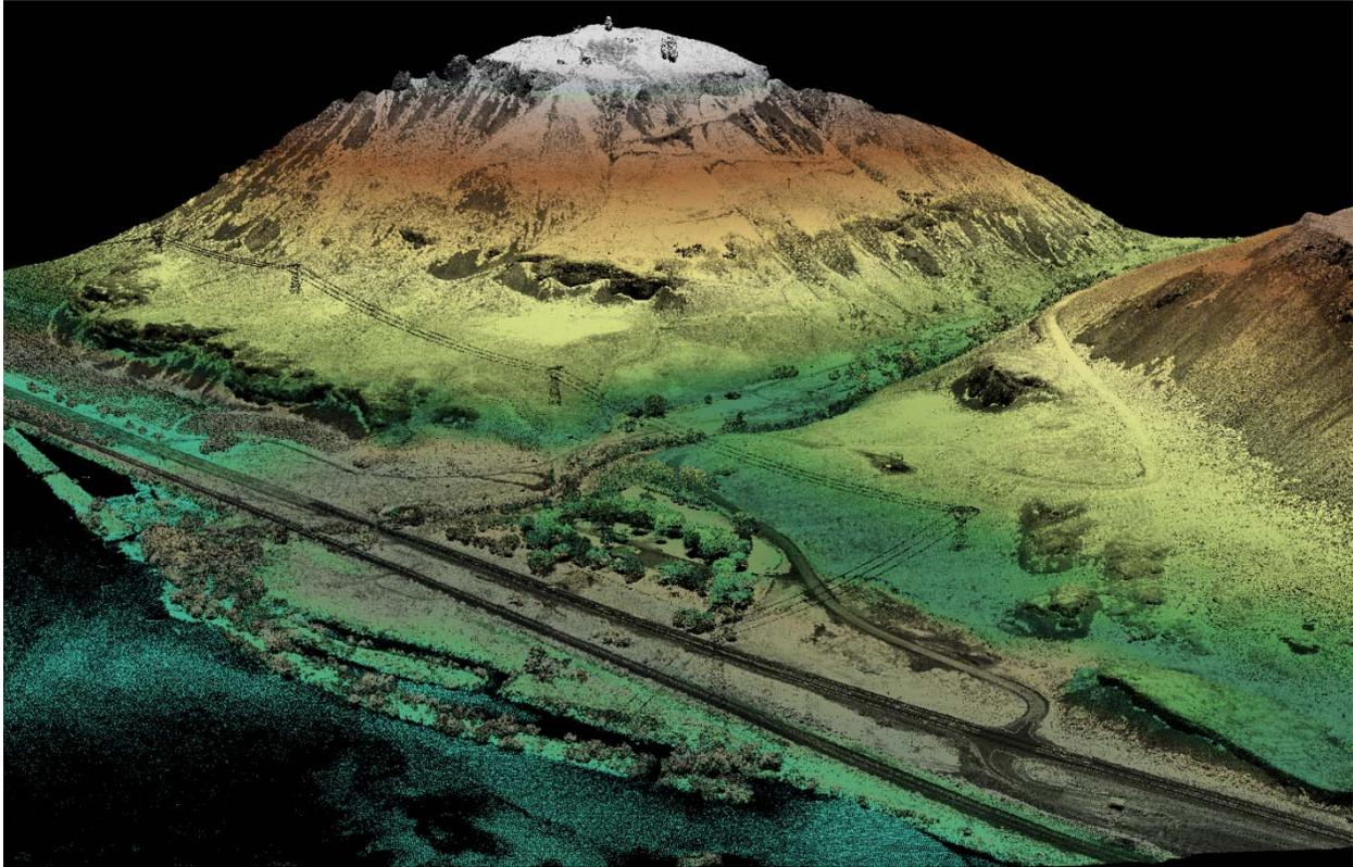
**Figure 12.** LiDAR derived point cloud image colored by elevation textured by intensity. Upstream view of Rock Island Creek showing both Washington State Route 28 and Rock Island grade (SW).
