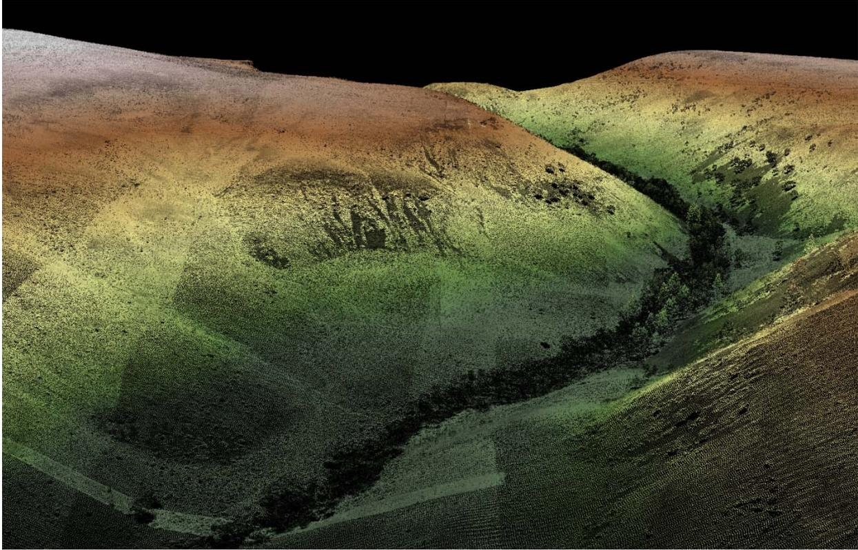
**Figure 11.** LiDAR derived point cloud image colored by elevation textured by intensity. Looking north at the confluence of the Columbia River and Rock Island Creek.
