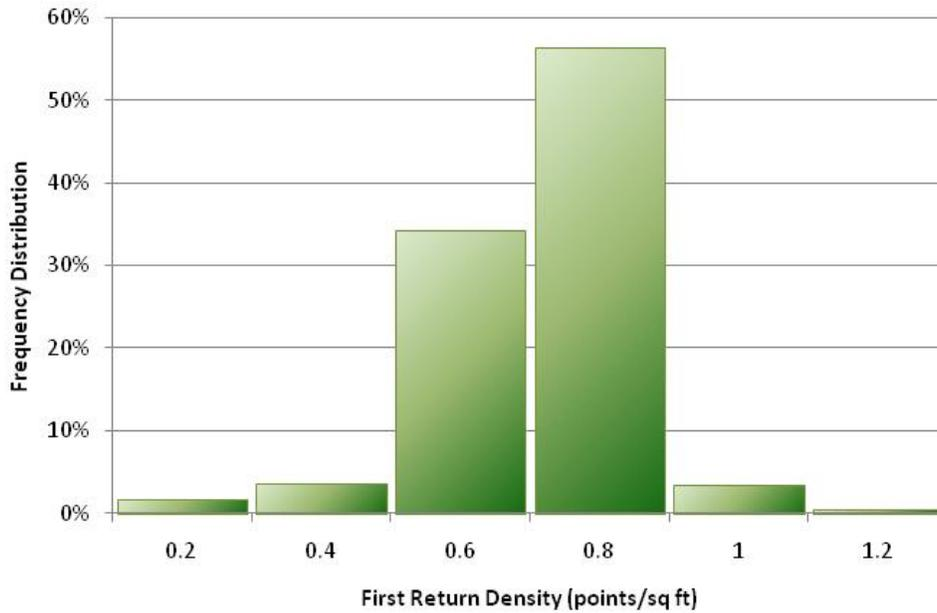
Figure 4. Density distribution for ground-classified laser points.
