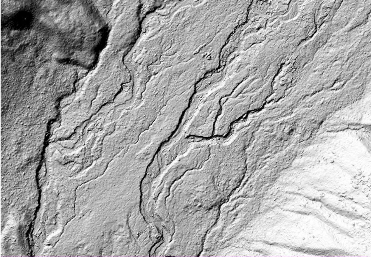
**Figure 6 - Shaded relief image of DEM made from the ground-classified LiDAR point cloud (NC2012) on the same portion of Kaust Creek. This DEM was created with a krigging interpolation algorithm. Ground class point density is still sub-optimal but improved from WS2008 to  $>1.2$  per  $m^2$**
