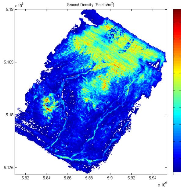
**Figure 8 - Ground class points per square meter.**
