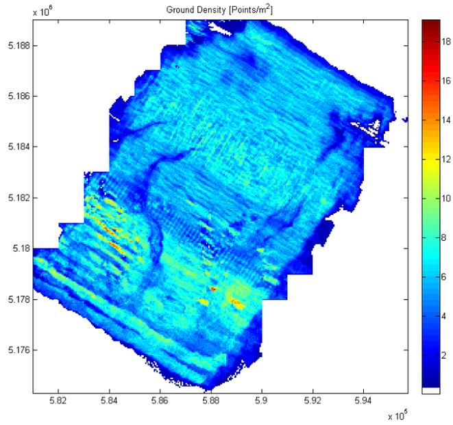
**Figure 7 - Laser shots fired per square meter.**
