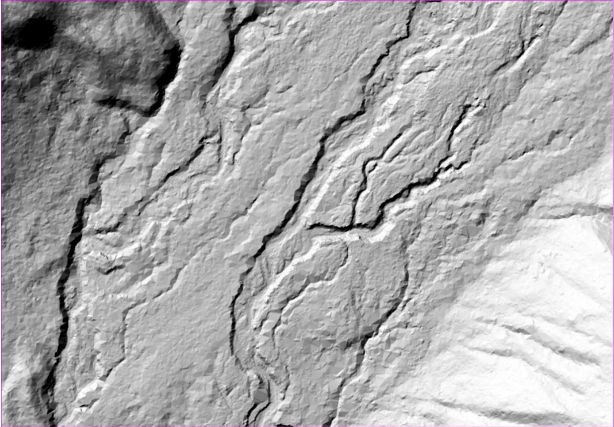
**Figure 5 - Shaded relief image of DEM made from the ground-classified LiDAR point cloud (WS2008) on the same portion of Kaust Creek. This DEM was created with a TIN interpolation algorithm. Ground class point density <math><1.0</math> per**
