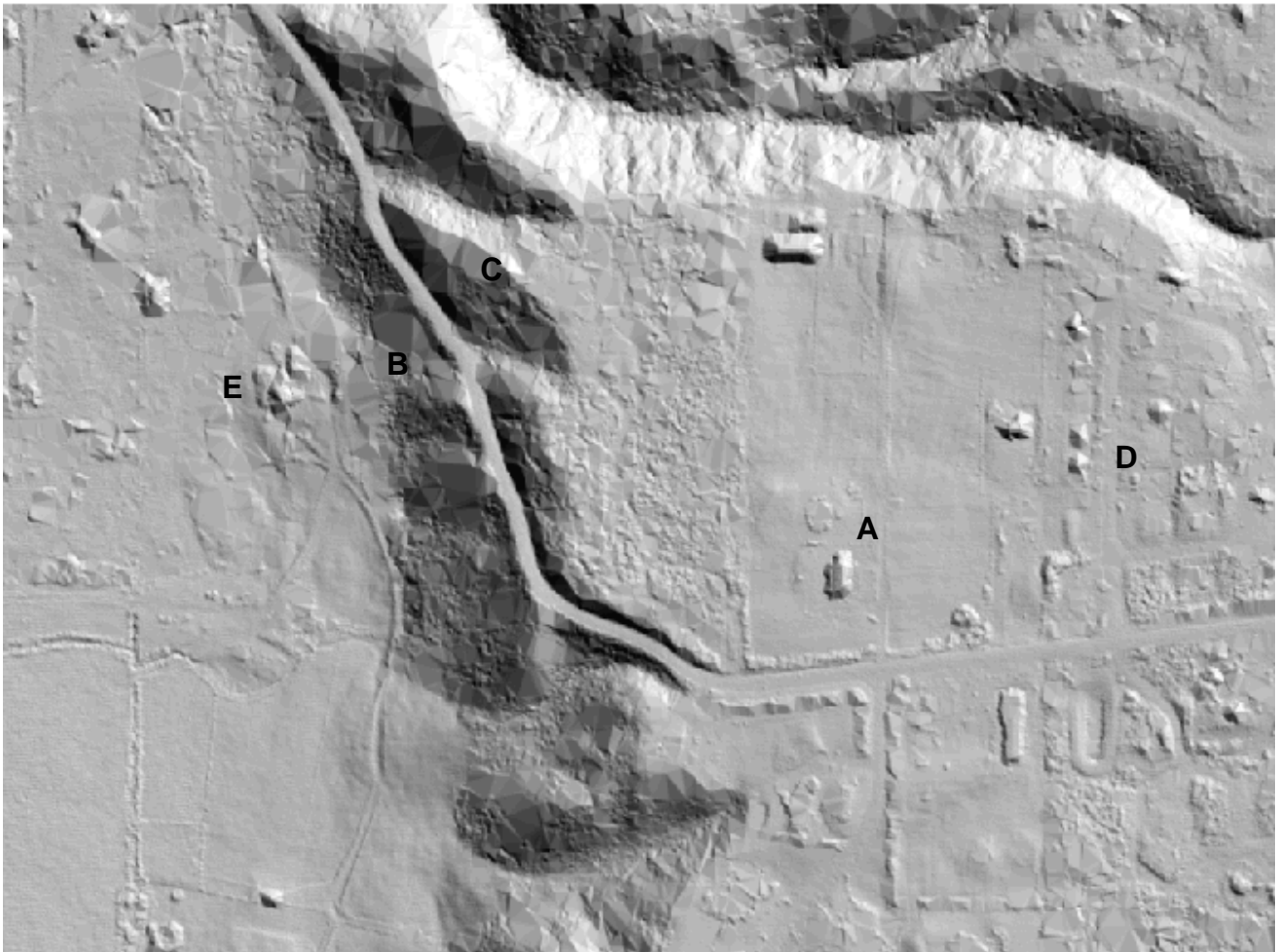
Figure 2. Surface model produced with despiking algorithm, same area as figure 1. Area shown includes about 2.7 \times 10^5 ground returns. See text for discussion.
