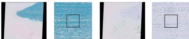
Lake Baikal error comparison. Both daytime images from southern part of Lake Baikal: R = 10, G = 12, B = 14. Good scene 12 Aug 2004, 6% bad pixels; bad scene 22 Jul 2002, 89% bad pixels. Note clouds in the "good" picture.
