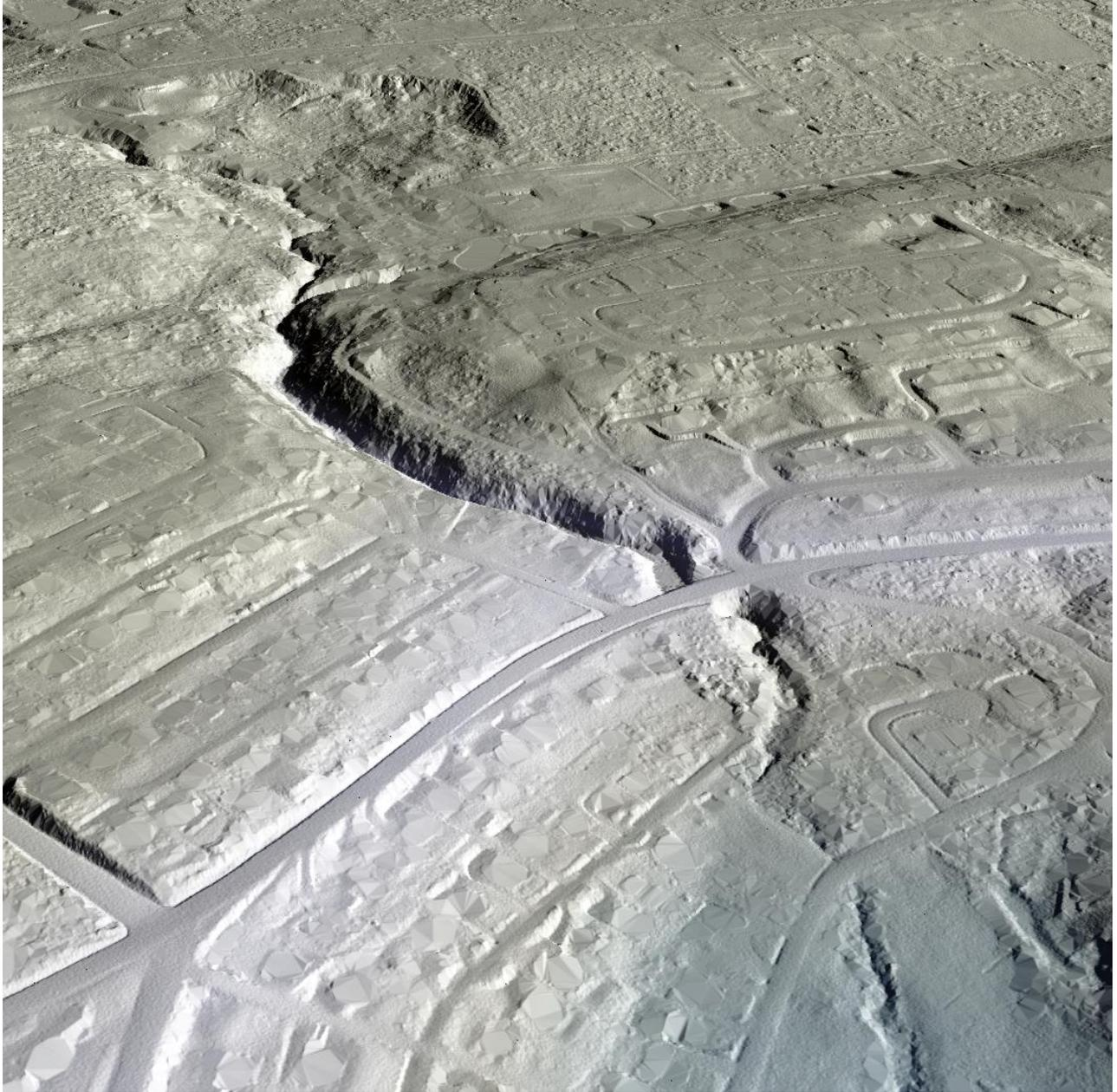
**Figure 10: A view looking west on Camano Island northwest of Dry Lake. The image was created from the bare earth model colored by elevation.**
