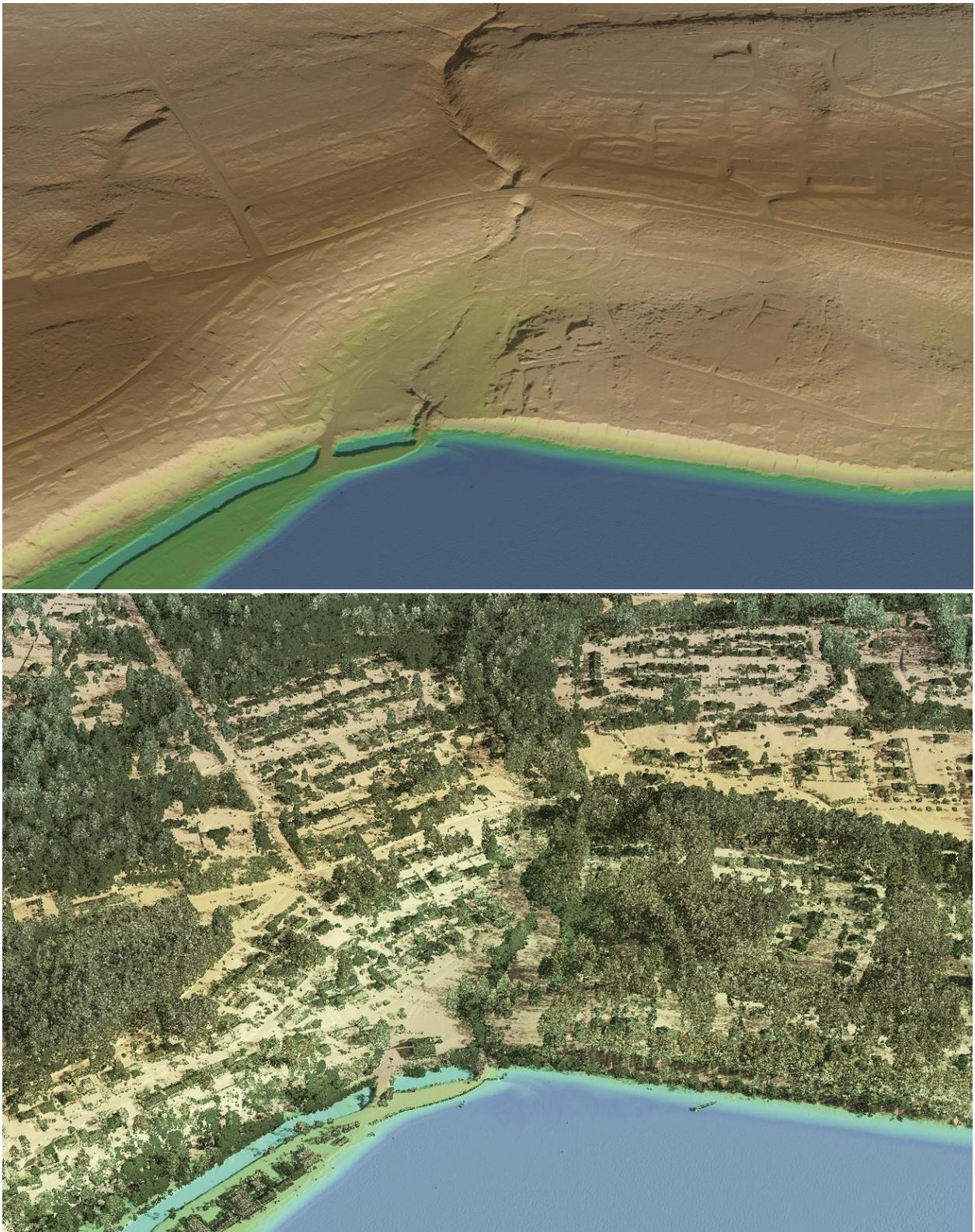
**Figure 13: A view looking east on Camano Island, northwest of Dry Lake. The top image was created from the bare earth model colored by elevation, and the bottom image is overlain with the highest hit LiDAR point cloud.**
