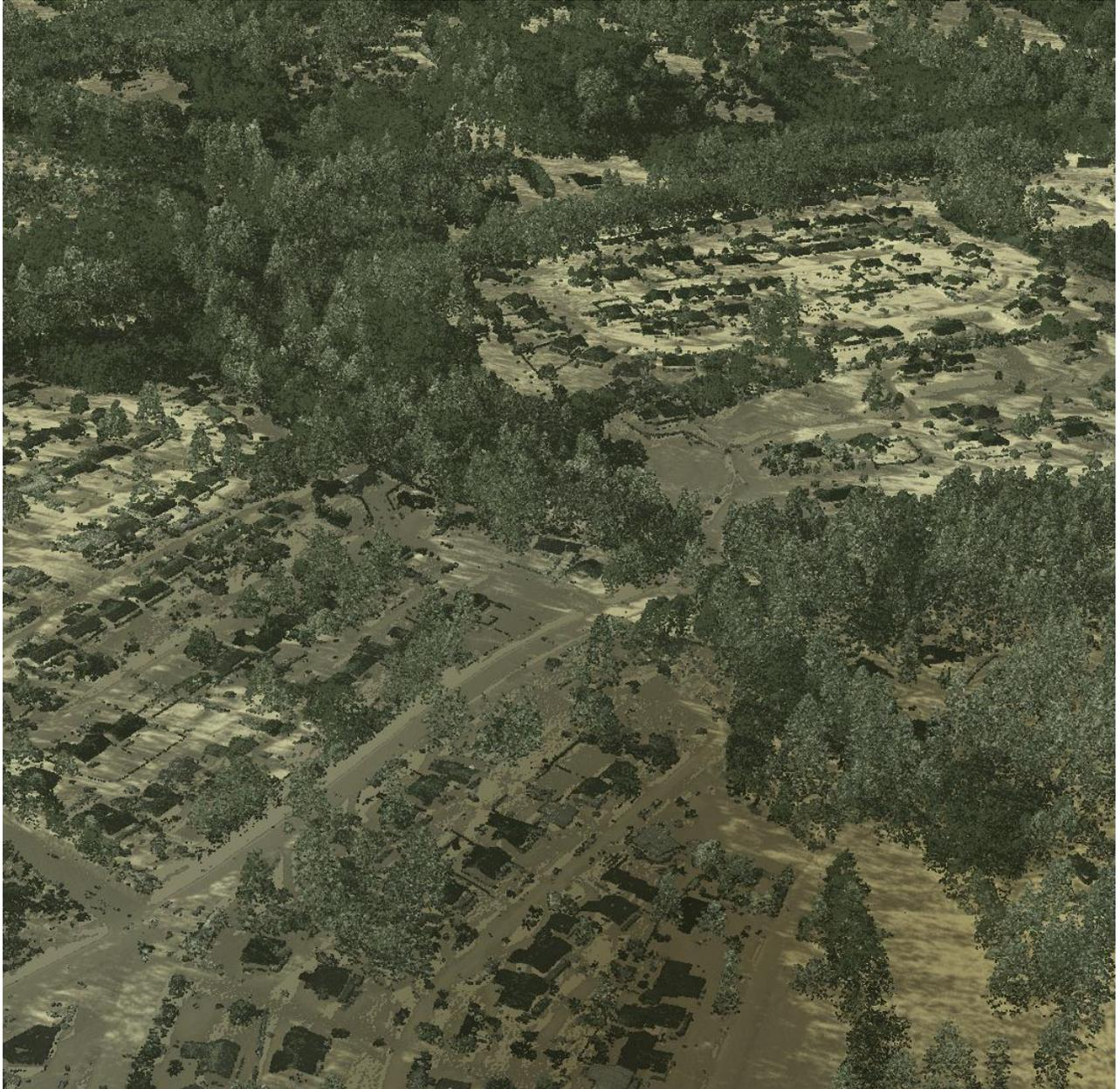
**Figure 11:** This image shows the same view as in Figure 10, but here the bare earth model is colored by elevation and overlain by the LiDAR highest hit point cloud.
