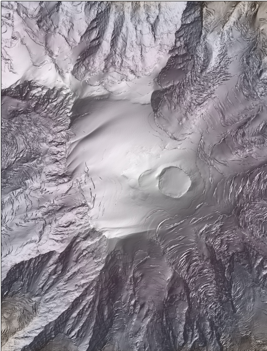
Figure 10. 2-d view of LiDAR derived bare earth surface: Mount Rainier Crater from above.
