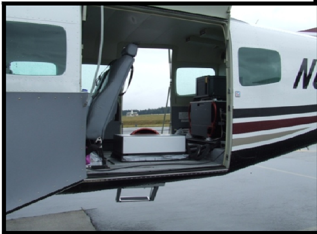
The Cessna Caravan is a stable platform, ideal for flying slow and low for high density projects. The Leica ALS50 sensor head installed in the Caravan is shown on the left.
