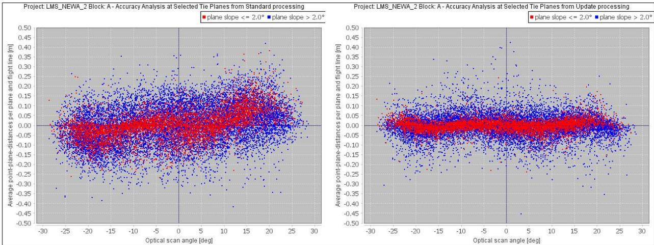
**Figure 7: Example of Zone 2A – mean values if the point to plane distances plotted over scan angle**
