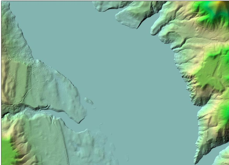
Figure 18: Example of Bare Earth DEM colored by height with hydro enforcement
