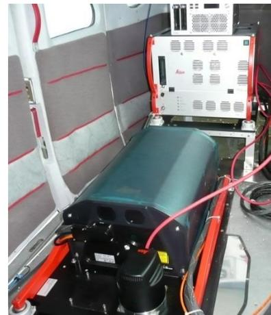
**Leica ALS70 LiDAR sensor**
