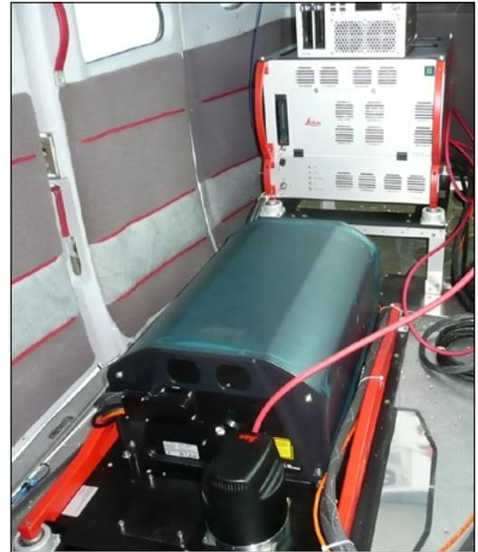
Leica ALS70 LiDAR sensor
