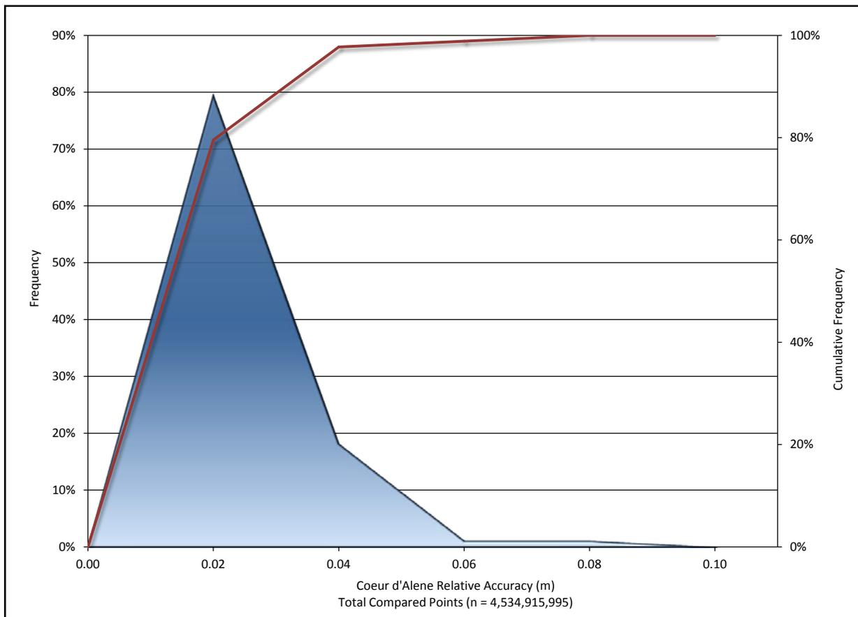
Figure 8: Frequency plot for relative vertical accuracy between Coeur d'Alene flightlines
