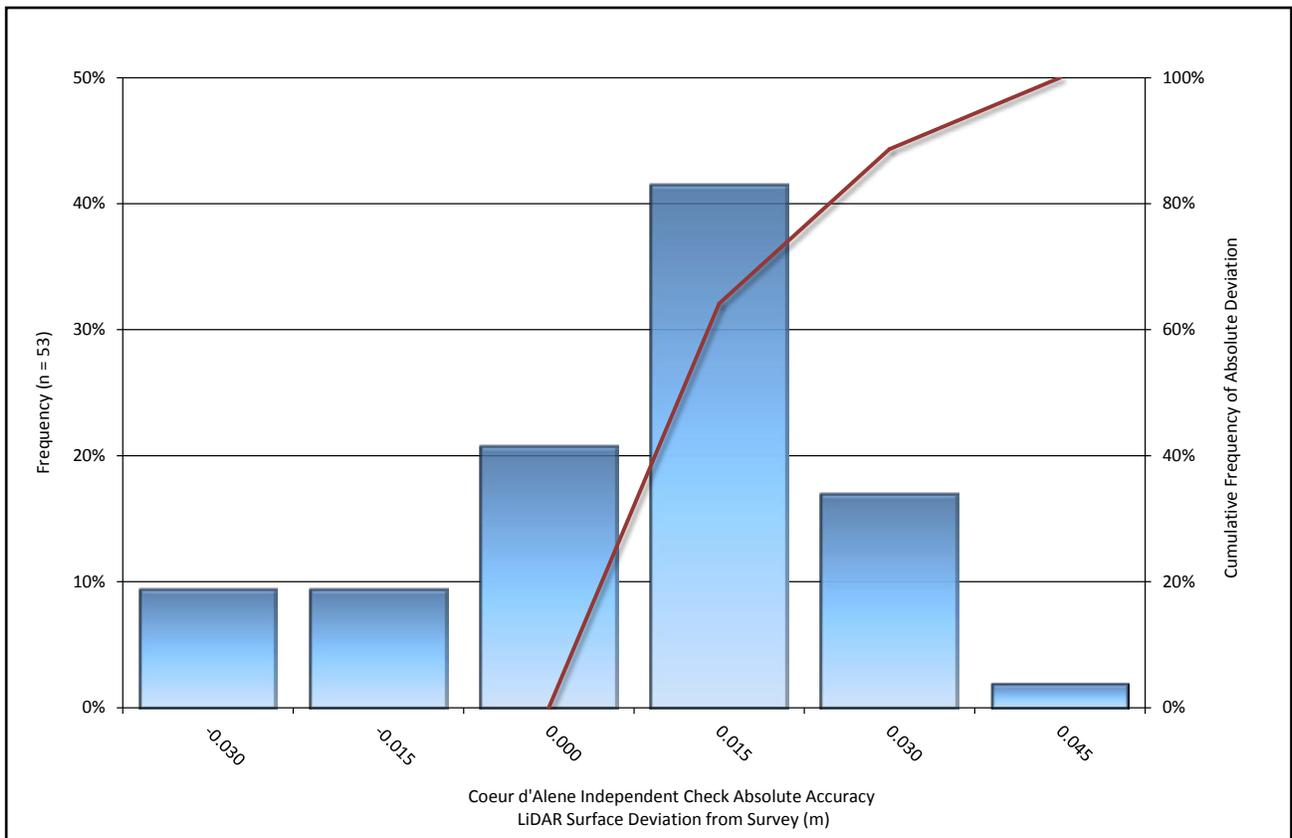
Figure 7: Frequency histogram for LiDAR surface deviation from reserved ground survey control point data.
