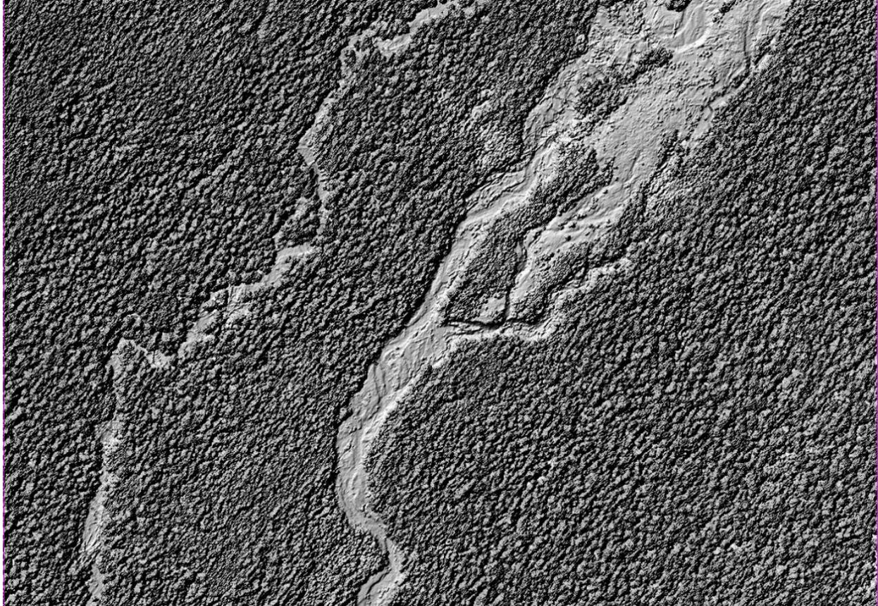
**Figure 4 - Shaded relief image of DEM made from the unclassified LiDAR point cloud (NC2012) on a portion of Kaust Creek. Native point density >8 per m<sup>2</sup>**
