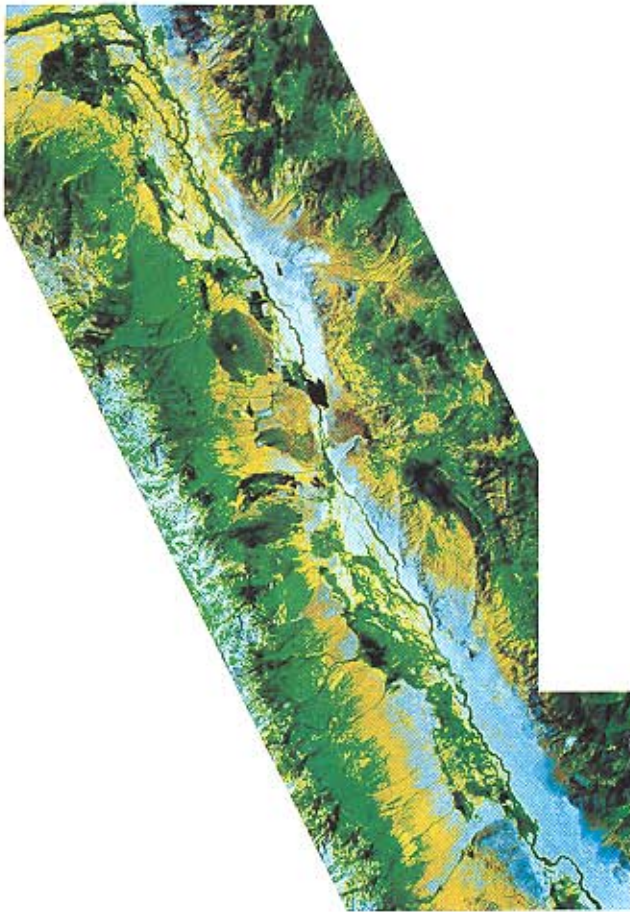
Figure 6. A vegetation map of Owens Valley derived from multispectral TM images. The image has been color-coded and calibrated by field cover estimates so that the vegetation cover is \leq 0.1 in gray areas, 0.11-0.3 in yellow areas, and > 0.30 in green areas. The intensity of the color is modulated by (1 - F_{\text{shade}}) . The Sierra Nevada on the left of the image is snow covered and the color codes are not applicable to this area.
